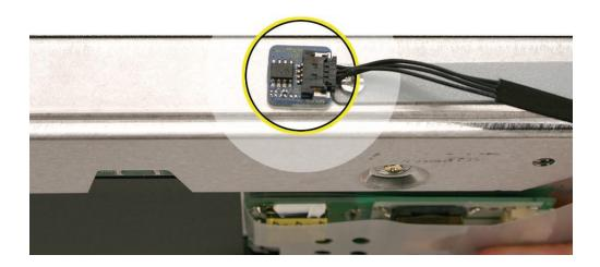
Route the cable along the right side on the back of the panel. Press the black sticky insulator over the top of the cable and the sensor. Replace any clear tape holding the cable in place on the panel..
